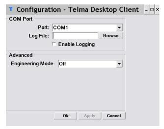
Open device manager on your computer. Click on START > RUN, type in devmgmt.msc and click OK or press ENTER. Check which COM port is assigned to the serial communications port or USB-to-serial adapter.
